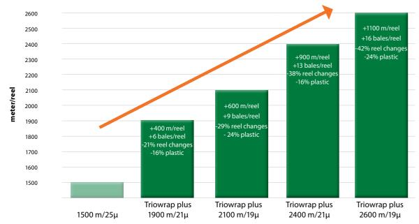
Based on: Round bale 1,20 m, 6 layers of film, 55 % overlap, 70 % pre stretch, when comparing to 1500 m/25 $\mu$  film.
